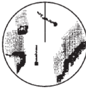
(b) Relative target trails Targets moving relative to own ship
